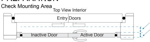
Allow 2-5/8" (67 mm) minimum space between entry door handle and mounting area to avoid hardware interference.
