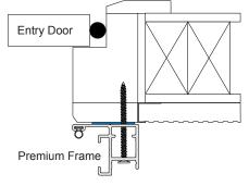
(5) Space remaining screws 3" (76 mm) from corners and 10" to 12" (254 to 305 mm) apart.
